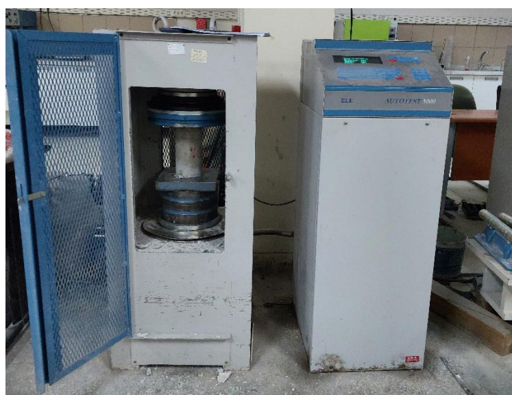
Fig. 3. Compressive strength test device used in this study
