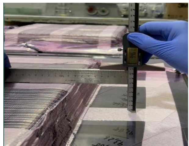
Fig. 1. Zones A, B, and C identified for thickness measurement under vacuum compaction
