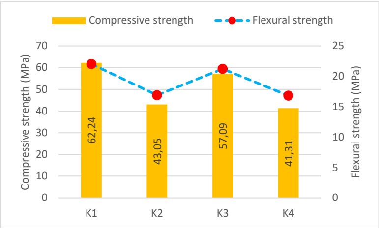
Fig. 4. Compressive and flexural strengths of SIFGEO
