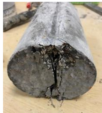
b) SCLC sample with macro steel fiber
