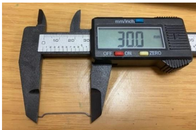
Fig. 2. The macro steel fiber used in this study
