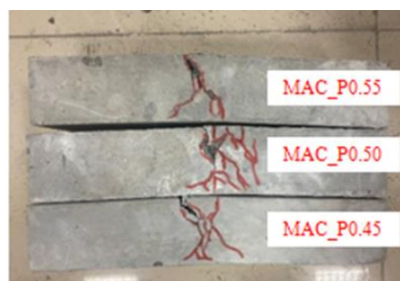
Fig. 21. The crack patterns of fiber-reinforced SCLC samples after the bending test
