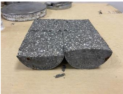
a) SCLC sample with no fiber
