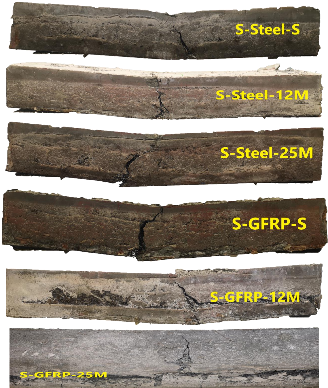
Fig. 14. Specimen photos after flexural test
