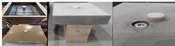
Fig. 7. A T-section glulam-concrete deconstructable connection [31]
