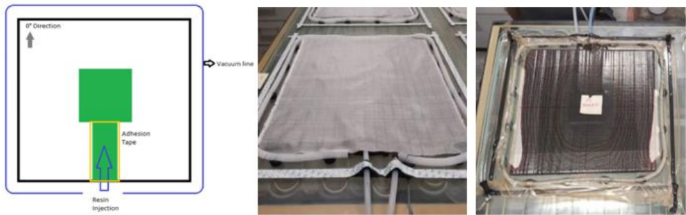
Fig. 4. Representation of permeability test system set-up
