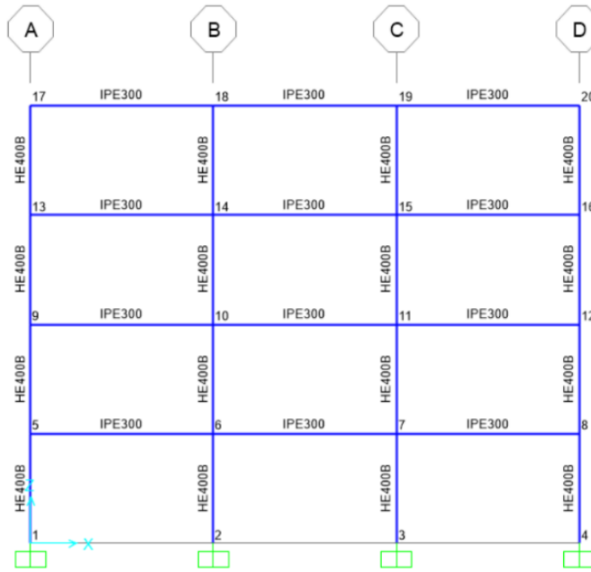
Fig. 3. 4-story plane steel frame model
