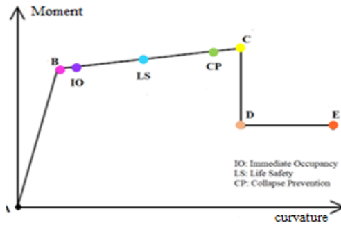
Fig. 4. Damage status ranges on the capacity curve
