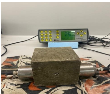
Fig. 6. Ultrasonic pulse device
