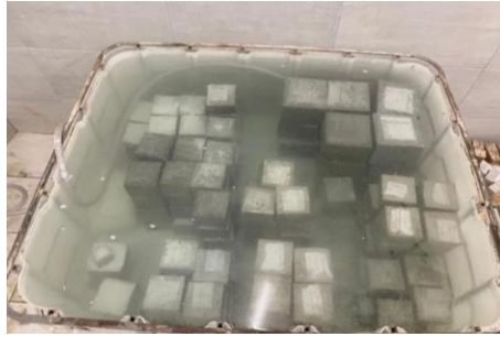
Fig. 3. Cured specimens in lime water
