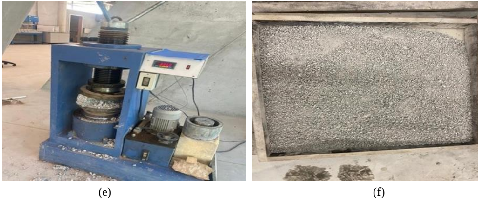
Fig. 2. (e) shows the recycled aggregate crushed using the compressive strength machine in the laboratory; (f) shows the recycled fine aggregate after crushed and sieved that passes through sieve 4.75 m
