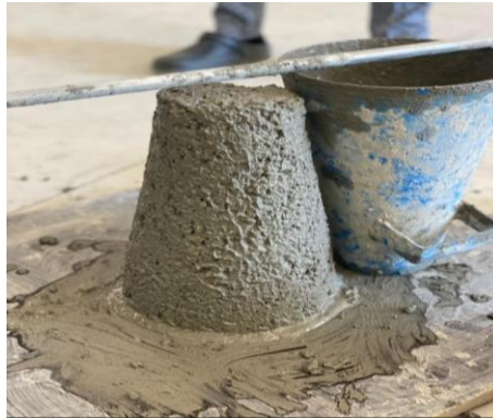
Fig. 4. A slump test of concrete mixture
