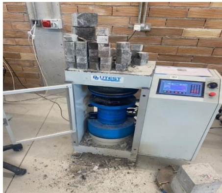
Fig. 5. A compressive strength machine
