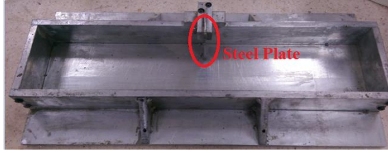
Fig. 4. Steel mold used for producing notched beam test specimens
