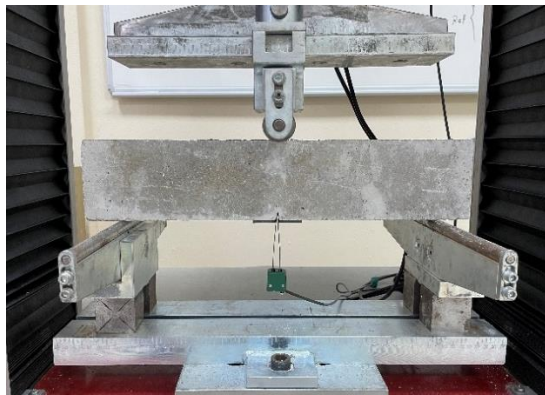
Fig. 5. Three-point bending test set-up
