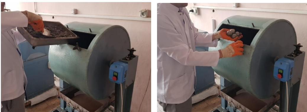
Fig. 8. Application of Los Angeles abrasion test
