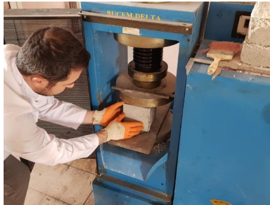
Fig. 9. Compressive strength test
