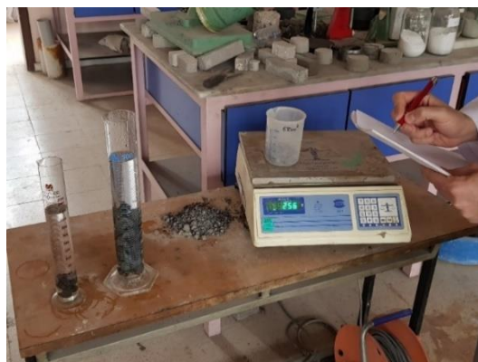
Fig. 7. Measurement of density
