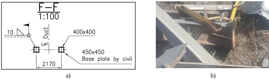
Fig. 17. (a) Column endplate (mechanical project), (b) View of column endplate after the collapse
