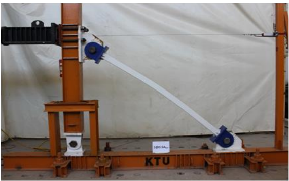
Fig. 4. The cyclic behavior of the C1 specimen until buckling
