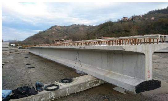
Fig. 3. Operational model testing of the PSC girder
