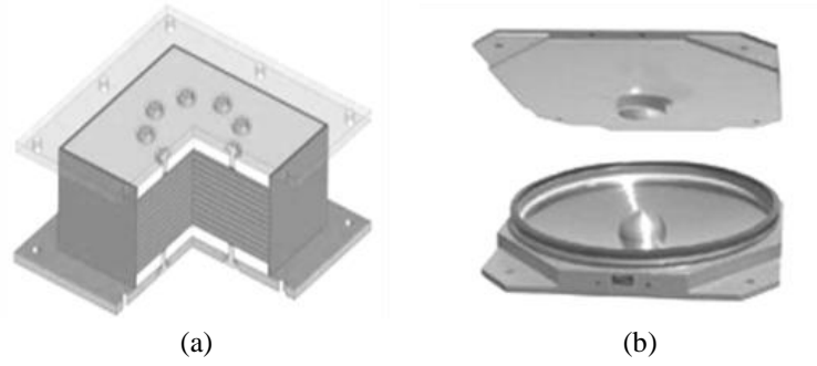
Fig. 2. a) Rubber and b) friction pendulum isolators
