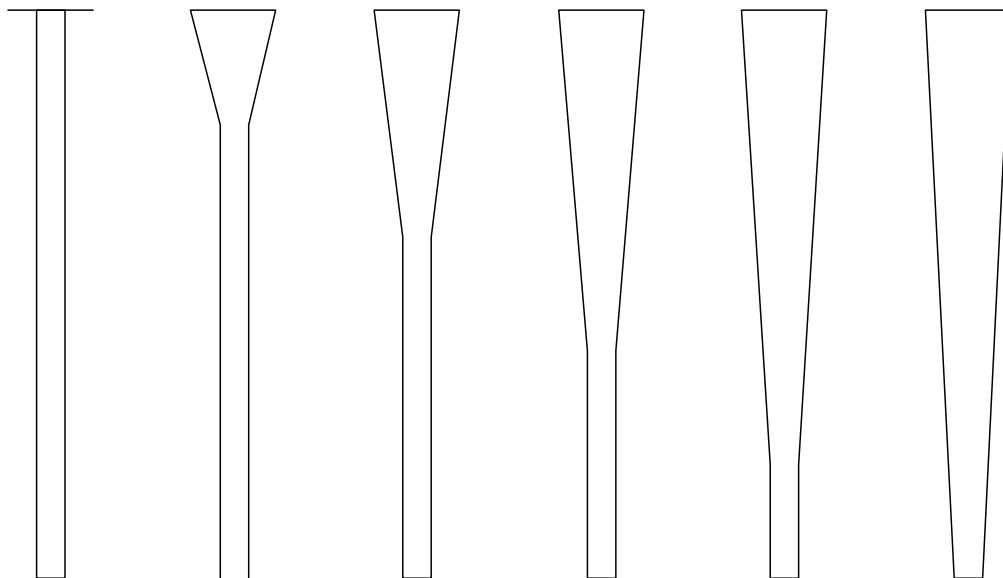
Fig. 4. Some examples of columns with variable cross-section according to L_1/L ratio
