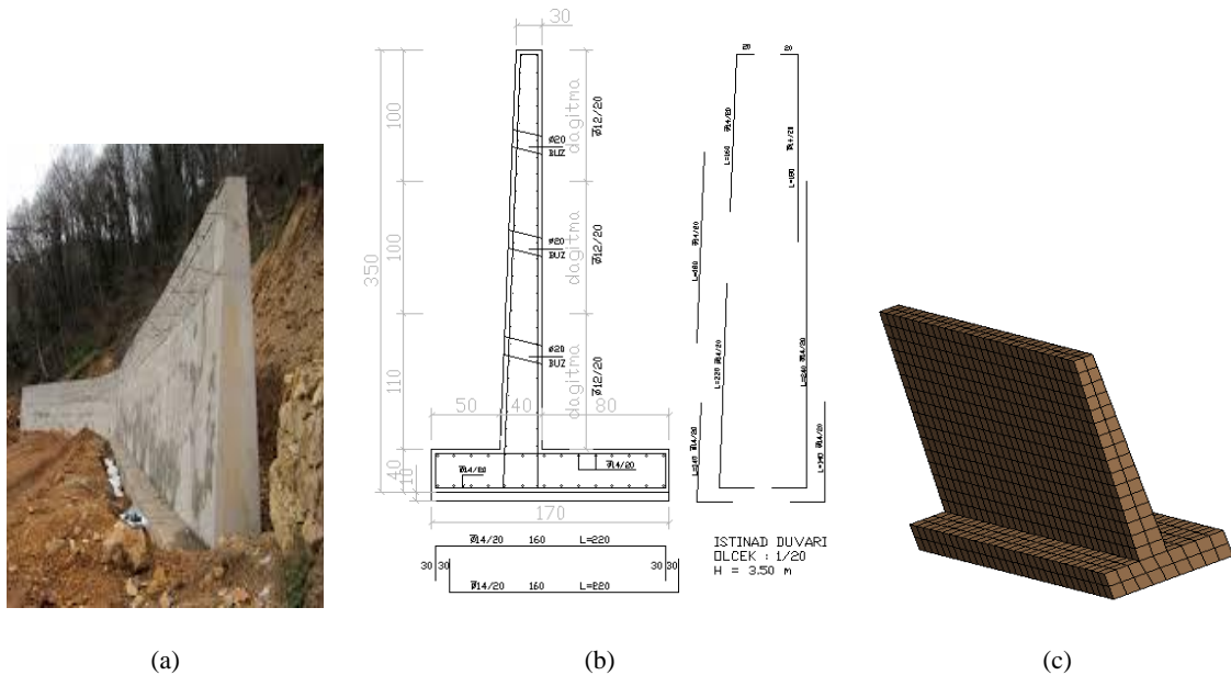
Fig. 4. (a) Photograph, (b) drawing and (c) finite element model of reinforcement retaining wall.
