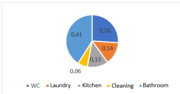
Fig. 3. Distribution of domestic water consumption (Referring to [27])
